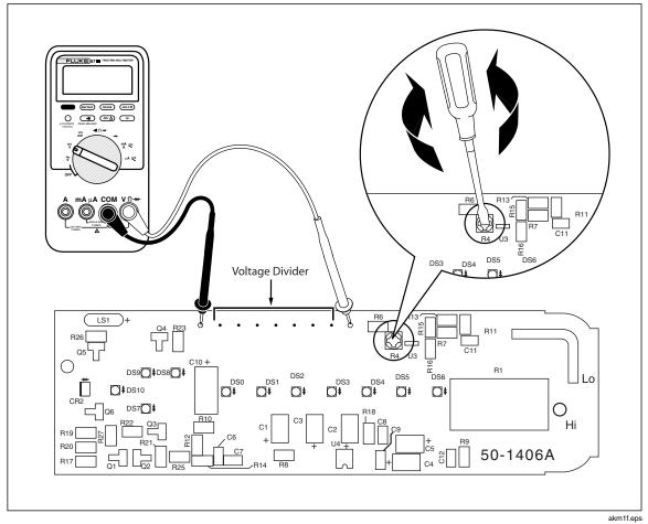
Figure 1. Calibration Adjustment Point
